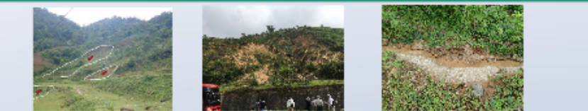
Fig.4: Landslide of weathered granitic rock (the Paleozoic) at area B in Fig.4. Left: Flow-type landslide (small landslide area about 10 m width and 30 m length). Middle: Slump-type landslide - a cluster of small landslides. Overall width about 250 m, length about 500 m. Right: Slide surface appearing at the toe of the landslide, which is made of the old landslide. (C: Direction of landslide movement)
